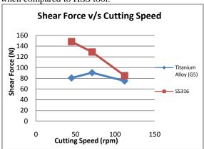
Graph 2: Shear force v/s Cutting speed
